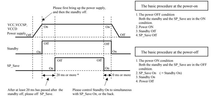
Note) \*: This IC contains the pre-charge circuit. It is time until each bias is stabilized from Standby Off. It depends for this time on the capacity value linked to a reference voltage terminal (VREF and VREFSP), and the capacity value and resistance linked to an input terminal (IN).
