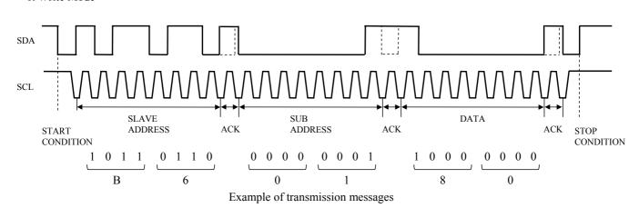
Two transmission messages (i.e., the SCL and SDA) are sent in synchronous serial transmission. The SCL is a clock with fixed frequency. The SDA indicates address data for the control of the reception side, and is sent in parallel in synchronization with the SCL. The data is transmitted in 8-bit, 3 octets (bytes) in principle, where every octet has an acknowledge bit. The following description provides information on the structure of the frame.
