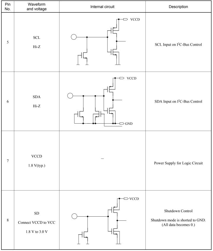
• I/O block circuit diagrams and pin function descriptions (continued) Note) The characteristics listed below are reference values based on the IC design and are not guaranteed.
