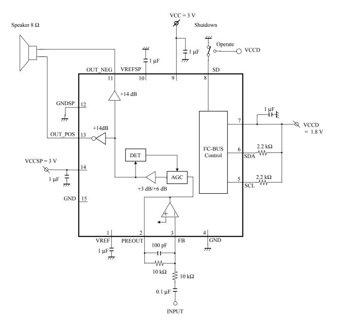
Note) 1. This circuit and these circuit constants show an example and do not guarantee the design as a mass-production set. 2. The threshold voltage at 8pin has the VCCD dependency.
